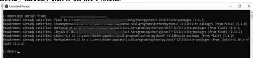
Fig 2. The Flask library installation process
